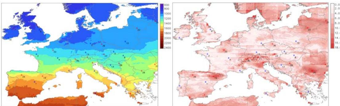
Fig. 1: Yearly sum of global horizontal irradiation, average of all five data bases [kWh/m<sup>2</sup>] (left), uncertainty at 95% confidence interval from the comparison of the five data bases. [%] (right).
