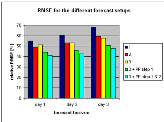
**Figure 2:** Error development over the three forecasting days. The RMSE increases stronger for the MM5 model approaches (1 and 2).
