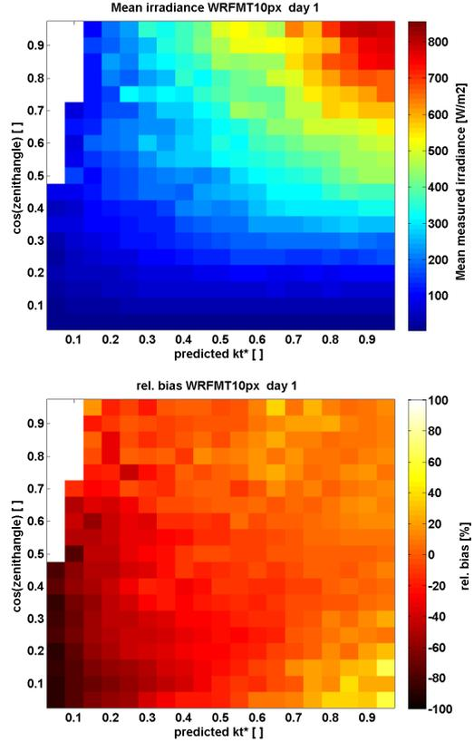
**Figure 1:** Mean (top) irradiance and relative bias (bottom) under a given zenith angle and a predicted clear sky index  $kt^*$ . These matrices are used as lookup tables for the bias correction in post-processing step 2.
